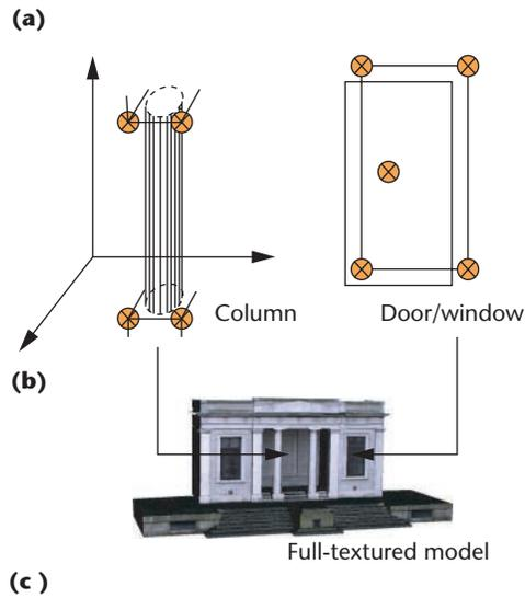
**3 Main steps for constructing architectural elements semiautomatically (column and window examples): (a) extract in multiple image steps, match, and compute seed points' 3D coordinates; (b) in 3D space, reconstruct the object from the seed points; and (c) create a full 3D model and project the new 3D points onto the image for texture mapping.**
