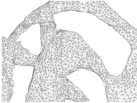
10 Close-up in the wire-frame model of part of the middle of a wheel (rose window).
