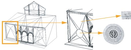
9 Integrating scanned and image-based models.
