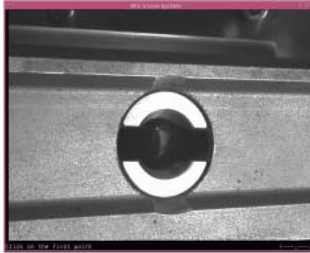
Figure 2 Planar feature of the bush inserted in the vessel stiffening ring
