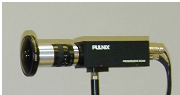
Figure 1: Nikon FC-E8 fish eye converter mounted on a Pulnix digital camera with a standard 12.5mm lens.
