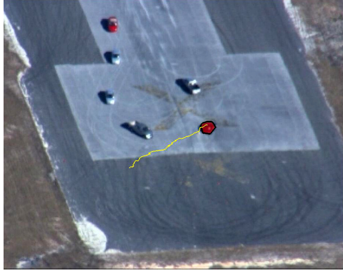
Figure 7. Convex hull and trajectory of a tracked object in sequence 1 (from the VIVID dataset).
