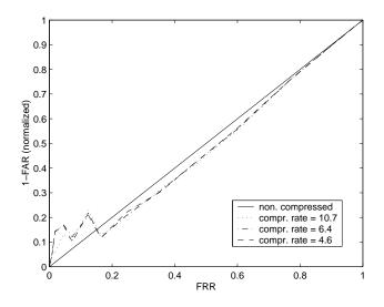
**Fig. 4**. Normalized ROC curves obtained from MIR matching (size 16x16 pixels) for wavelet-compressed and decompressed MIR's. Normalization was performed with the ROC curve of the noncompressed data (shown as straight line) as reference curve. For a better visibility deviations from the reference curve are magnified by a factor of 10.
