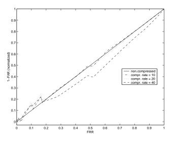
**Fig. 3**. Normalized ROC curves obtained from MIR matching (size: 16x16 pixels) for PCT-compressed and decompressed MIR's. Normalization was performed with the ROC curve of the non-compressed data (shown as straight line) as reference curve. For a better visibility deviations from the reference curve are magnified by a factor of 5.
