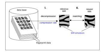
**Fig. 1**. The matching process with two independent subprocesses with one parameter.
