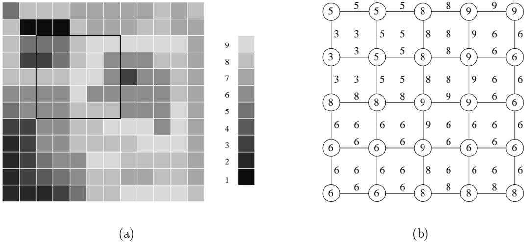
**Figure 1:** (a) The gray levels of the pixels. (b) The image graph of the marked sub-image (inside the black border), where the vertices are represented as circles. The numbers in the vertices and at the edges indicate the vertex values and the edge values of the image graph. The numbers in the middle of the square faces refer to the vertices of the dual graph.
