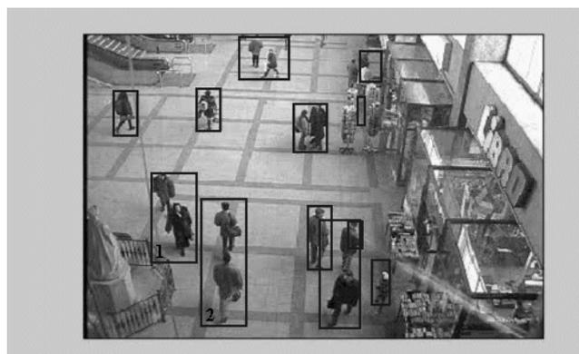
**Figure 6:** *Blob detection: The sizes of the bounding boxes of blobs 1 and 2 indicate that more than a single person is contained. Equation (11) allows the computation of the maximum number of people for every single blob.*
