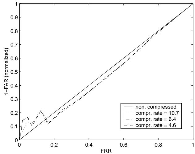
**Fig. 4.** Normalized ROC curves obtained from MIR matching (size 16x16 pixels) for wavelet-compressed and decompressed MIR's. Normalization was performed with the ROC curve of the noncompressed data (shown as straight line) as reference curve. For a better visibility deviations from the reference curve are magnified by a factor of 10.
