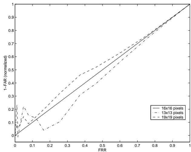
**Fig. 5.** Normalized ROC curves obtained from matching of non-compressed MIR's of different sizes (13x13, 16x16, and 19x19 pixels). Normalization was performed with the ROC curve of MIR data of size 16x16 (shown as straight line) as reference curve. For a better visibility deviations from the reference curve are magnified by a factor of 10.
