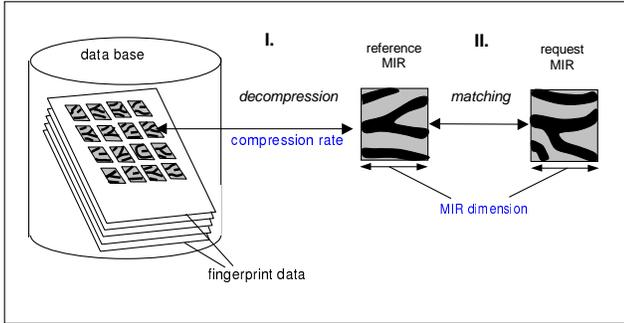
**Fig. 1.** The matching process with two independent sub-processes with one parameter.
