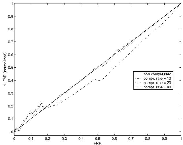
**Fig. 3.** Normalized ROC curves obtained from MIR matching (size: 16x16 pixels) for PCT-compressed and decompressed MIR's. Normalization was performed with the ROC curve of the non-compressed data (shown as straight line) as reference curve. For a better visibility deviations from the reference curve are magnified by a factor of 5.
