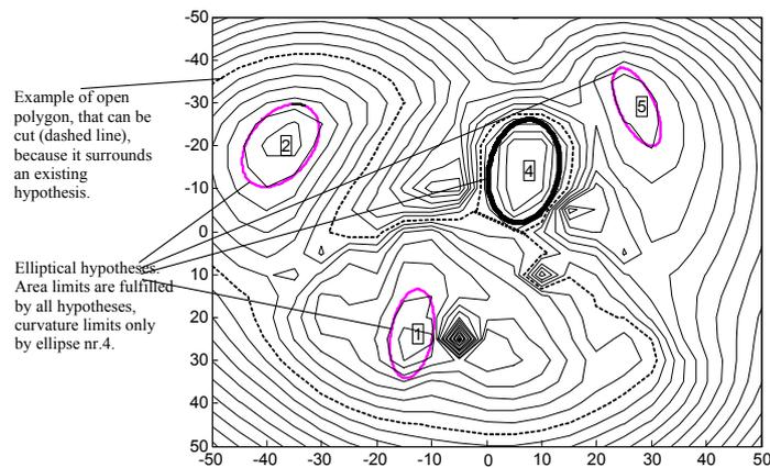
**Fig.1.:** Contour plot of reconstructed surface with ellipse hypotheses. Darker lines are contours that are close to the camera. Dashed line shows an example of an open polygon and a cut of an elliptical part of the polygon. Ellipses show hypothesis, dark ellipse fulfils all head conditions, bright ellipses violates curvature condition.
