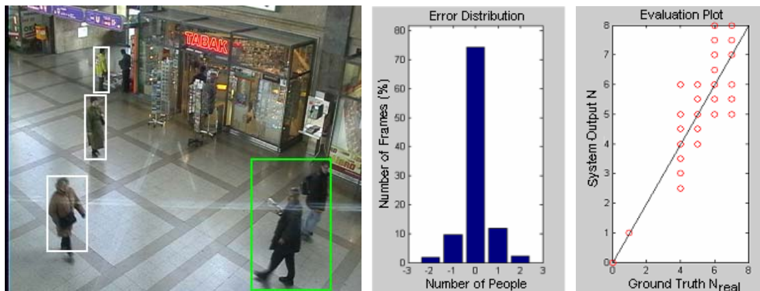
Figure 2: Blobs, error distribution and evaluation plot of the sample video ‘Shopping Mall’
