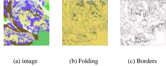
Fig. 2. Folding (b) of a combinatorial pyramid encoding the connected components of image (a). The borders of the partition are represented in (c).
