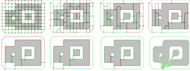
Figure 4: The boundary graphs of all the levels of an irregular graph pyramid (level 0 on the top-left) and the homology-generator level (on the bottom-right). Removed edges in black, contracted edges in red and surviving edges in green.
