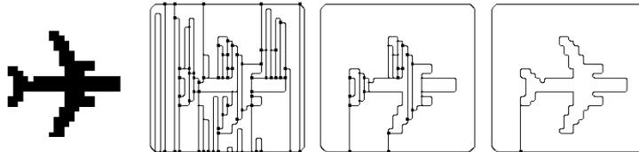
Figure 2: A digital image  $I$ , the boundary graphs of levels 6, 10, and the last one of an irregular graph pyramid of  $I$ .
