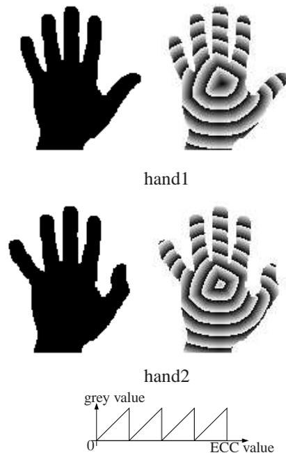
**Figure 1:** Eccentricity transform of two shapes from [19]. The grayvalues are the eccentricity value modulo a constant.
