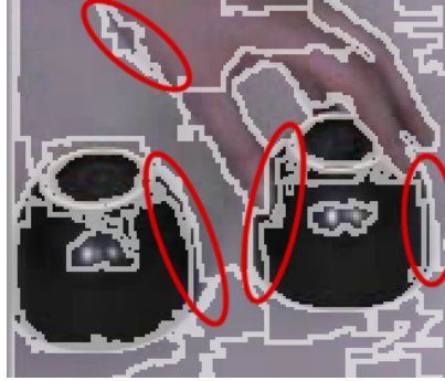
Figure 6: Elements covering object borders make edge detection difficult.
