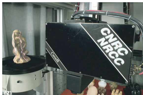
B Autosynchronized scanning configuration. (1) A dual mirror configuration. (2) A high-resolution sensor using a polychromatic laser for color measurement.
