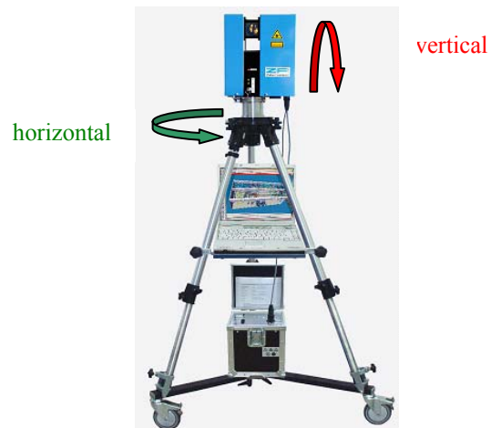
Fig. 3: Panoramic view scanner (IMAGER 5003)
