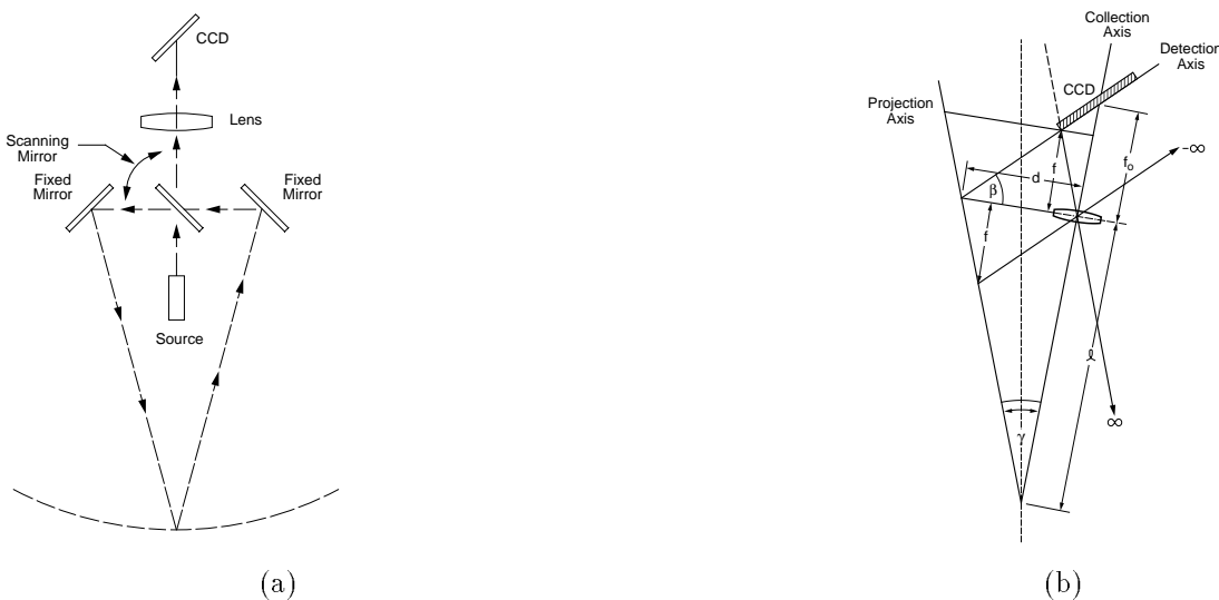
Figure 2: Auto-synchronized scanner approach: (a) with double-coated mirror, (b) Scheimpflug geometry.
