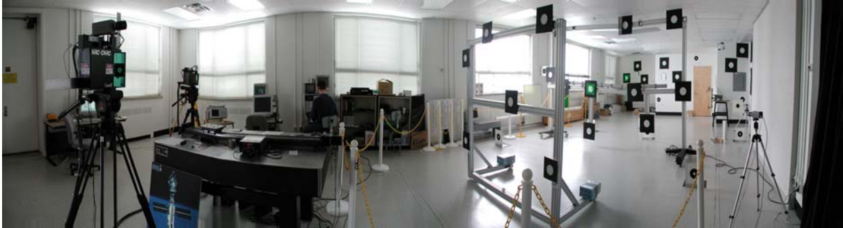
Figure 9. Experimental setup used to verify the accuracy of the tracking system. The three groups of targets are used to calculate their relative poses; the laser scanner camera is moved to view the targets from different angles.
