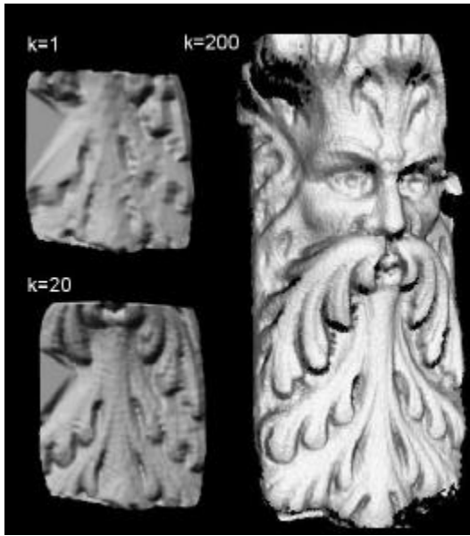
Figure 6: Multi-resolution model of Figure 5. From the initial low-resolution and distorted model \hat{\mathbf{m}}_0 to the more refined version \hat{\mathbf{m}}_k (respectively K=1, 20 , and 200, N=128 ).
