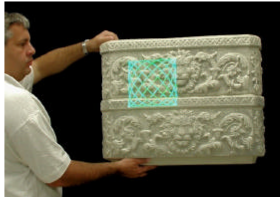
Figure 2: Hand-held acquisition using fast Lissajous scanning patterns and real-time tracking using the 3D range data. External constraints imposed in Figure 1 or by using external trackers are completely removed; no external equipment is needed. This is one of the experimental configurations we used during this work, the exactly equivalent opposite being holding the 3D camera.
