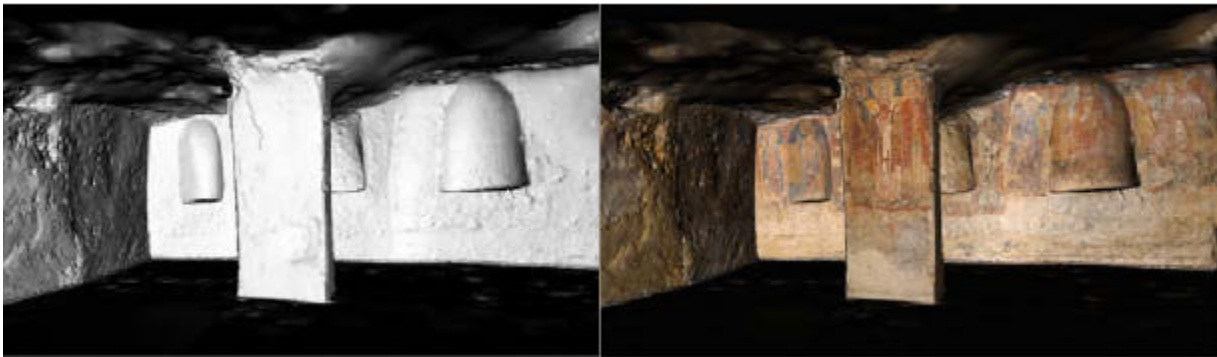
Figure 3: Texture mapping results of a Byzantine Crypt by combining Laser Scanner Data (left) and high-resolution color textures mapped on the model of the Crypt (from Beraldin, 2002).
