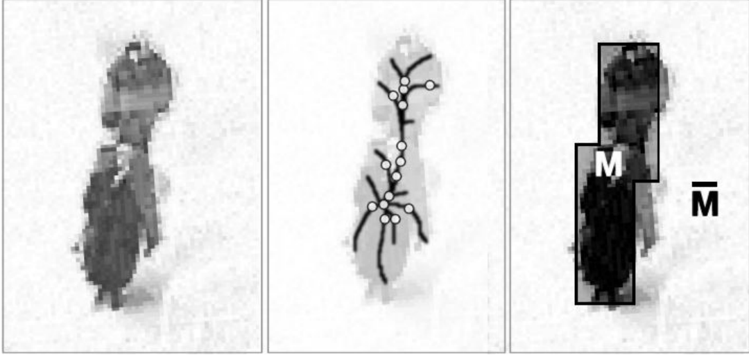
Figure 1: Example frame illustrating the approach to search for the most probable configuration of two humans in the presence of occlusion. Left: Occlusion between two humans shown in the inverted difference image. Center: Mode seeking is performed starting from a set of sample points. Obtained path points (shown as dots) represent possible locations of a human. Right: the optimal configuration of two objects for the given image region.
