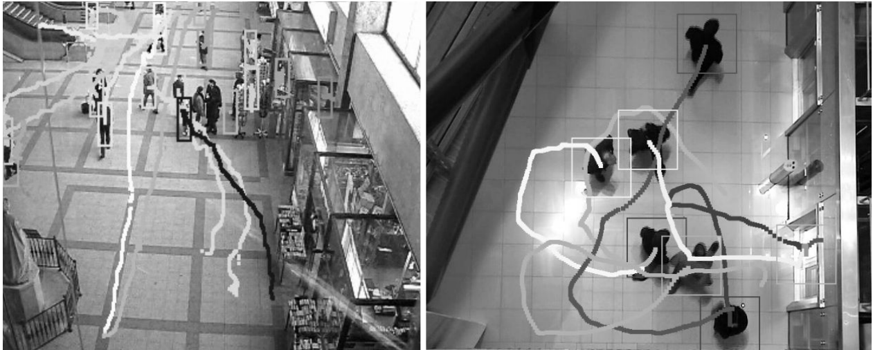
Figure 2: Tracking results obtained using the proposed occlusion handling scheme. (a) Example frame showing tracking results for Sequence A containing people moving along relatively straight trajectories. (b) Obtained tracks for a scene of Sequence B viewed by a top-mount camera. Humans in this scene perform more irregular movements.
