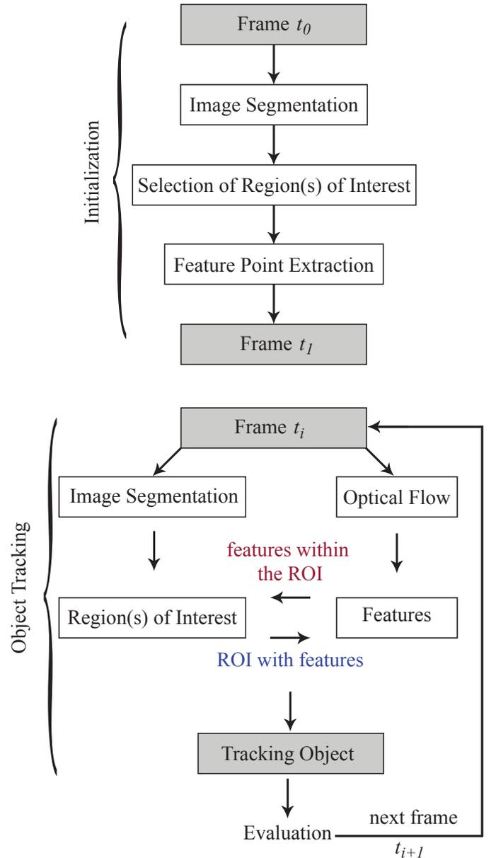
Figure 1: Workflow of the tracking Algorithm 2.
