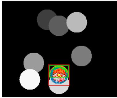
**Figure 3:** The tracked (partly occluded) ball in the MUSCLE benchmark. Green are found feature points, blue estimated feature points and red lost feature points. The orange color shows our segmented tracking object with its green bounding box. The red bounding box is from the ground truth data and incorrect, since it does not honor the occlusion of the object.
