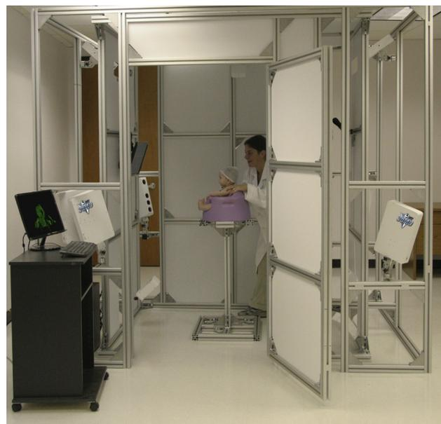
Figure 1 3dMDflex system (Courtesy of 3dMD, Atlanta, Georgia, USA; with permission).
