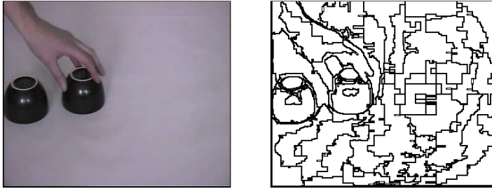
Figure 5: An image and the result of segmenting it with the MST algorithm [9].
