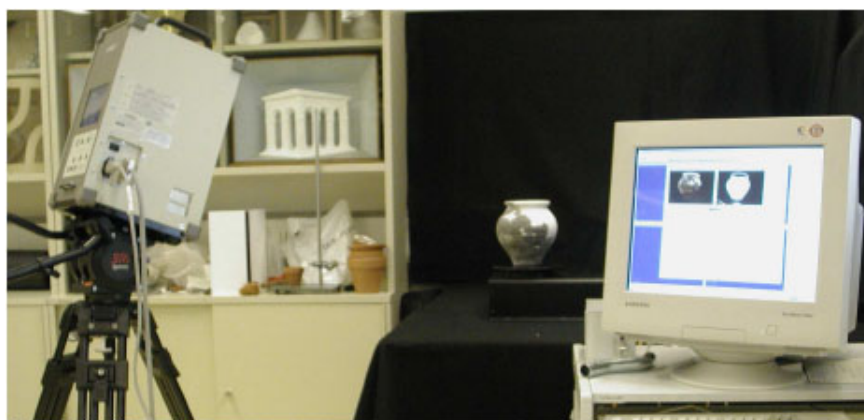
Figure 4: Scanning of a vessel. Left: 3d scanner focussing the object on the object. The object is on an automatic turntable connected to the computer on the right. The scanner and the turntable are controlled by the computer. The 3d scan data is registered automatically based on the information from the turntable. From: [3]
