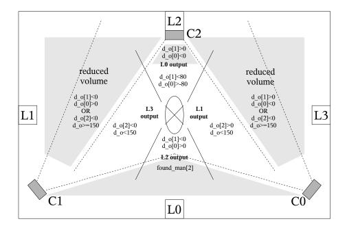
Figure 2: Diagram summarizing the conditions for the generation of each possible output. (Note: d\_o and d\_o[n] refer to the respective distance\_obs parameters in the code.)
