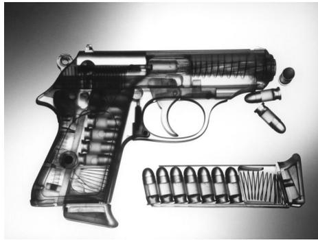
**Fig. 3.** Example of a resulting image for a pistol scanned by an industrial X-ray scanner [13]
