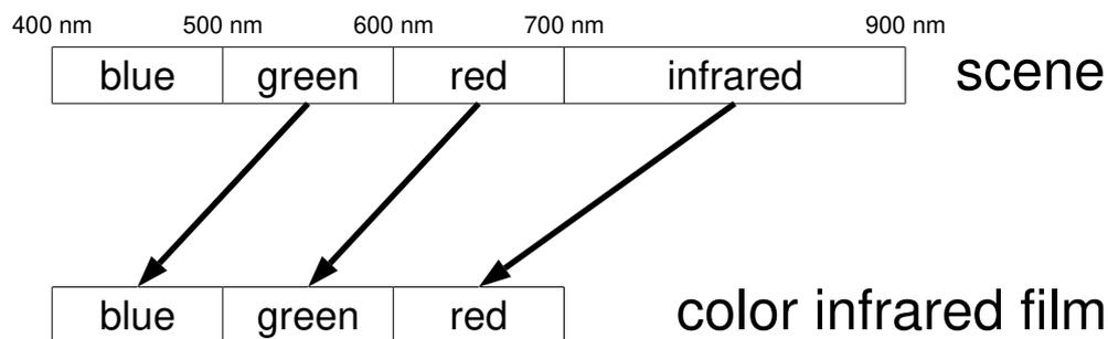
Figure 1: Spectral characteristics of color infrared film
