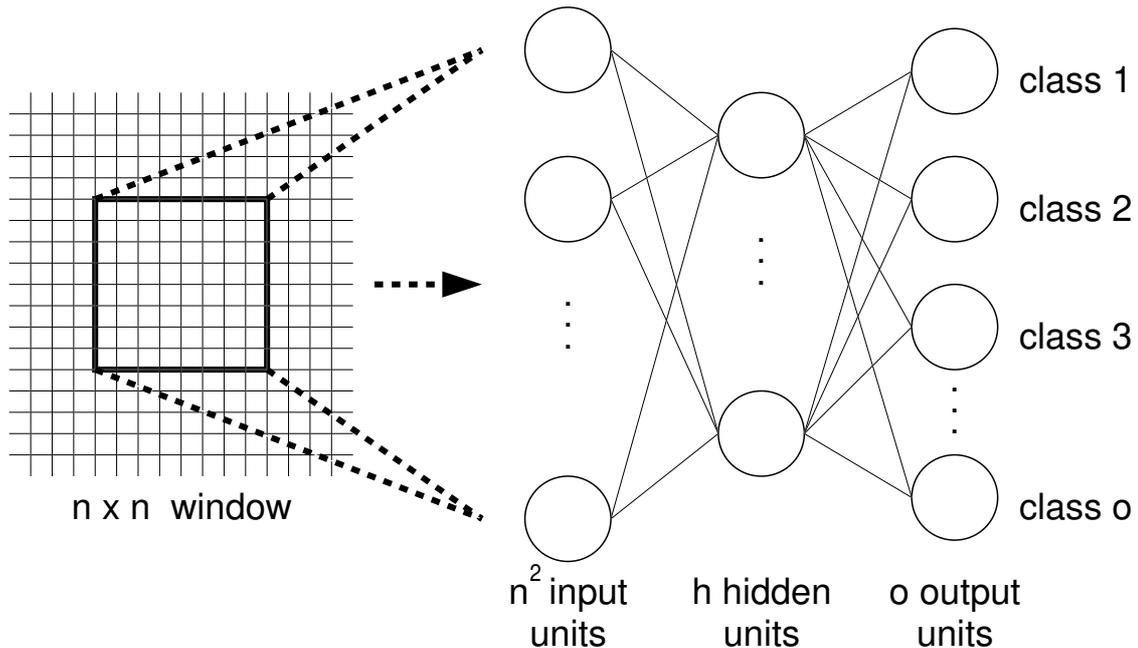
Figure 6: A feedforward neural network for image analysis
