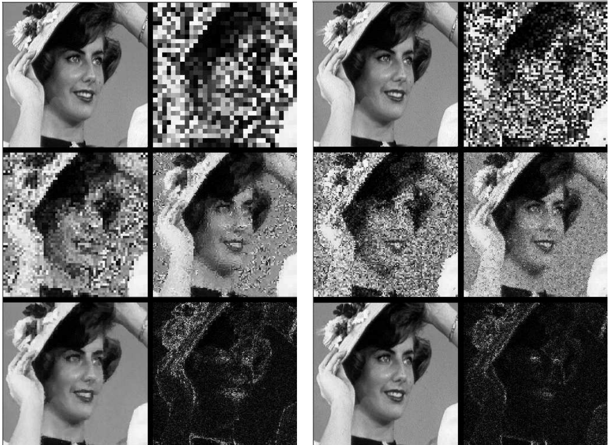
(a) 1024 non-overlapping squares of size 8 * 8 in partition R. Compression ratio = 20.4:1, PSNR = 27.2 dB.
