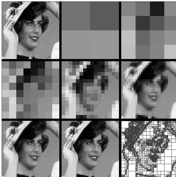
Figure 5: Quadtree evolution. The final Quadtree has 5719 squares.
