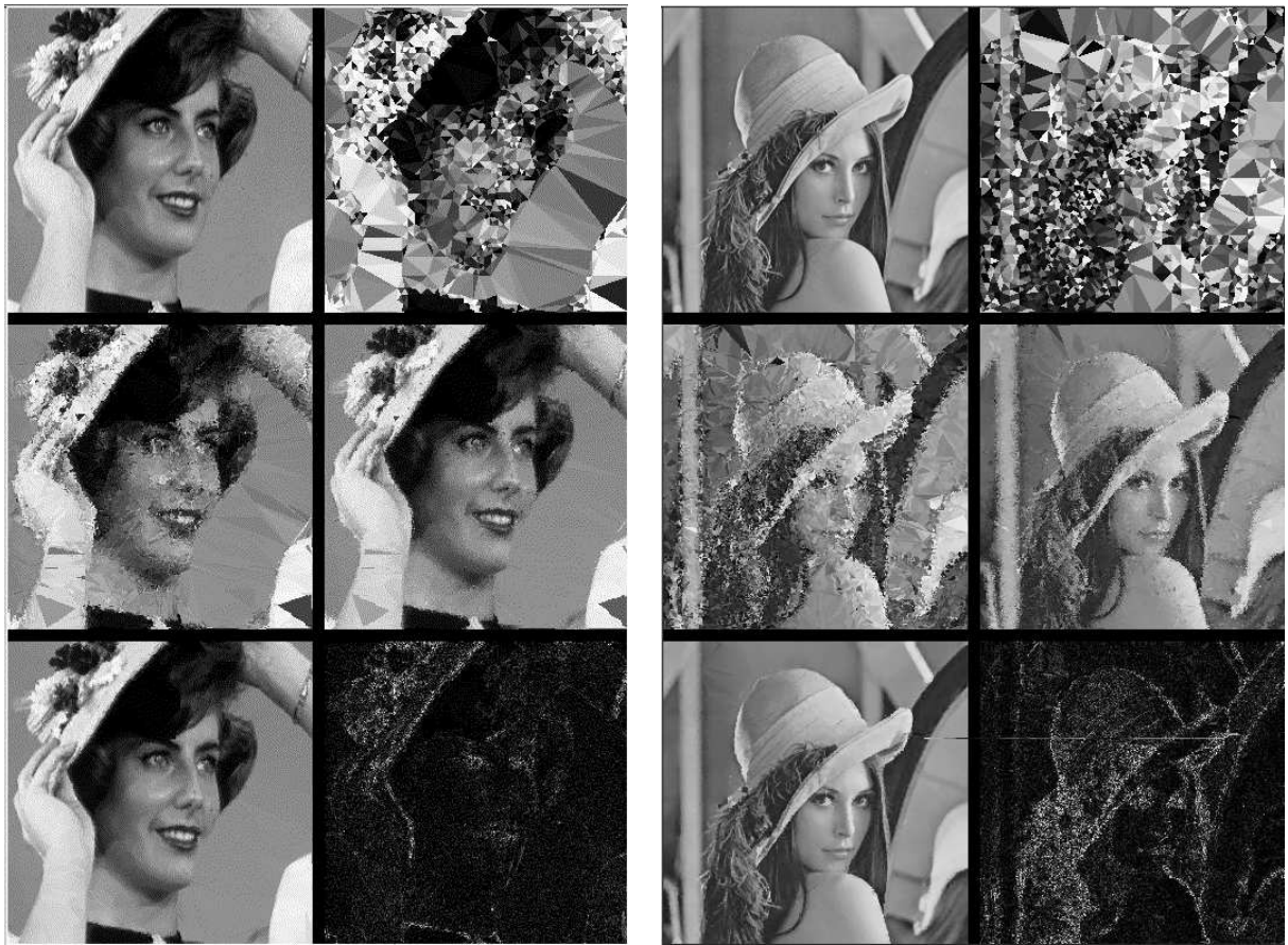
(a) Partition R of figure 7.c : Compression ratio = 9.5:1, PSNR = 30 dB.
