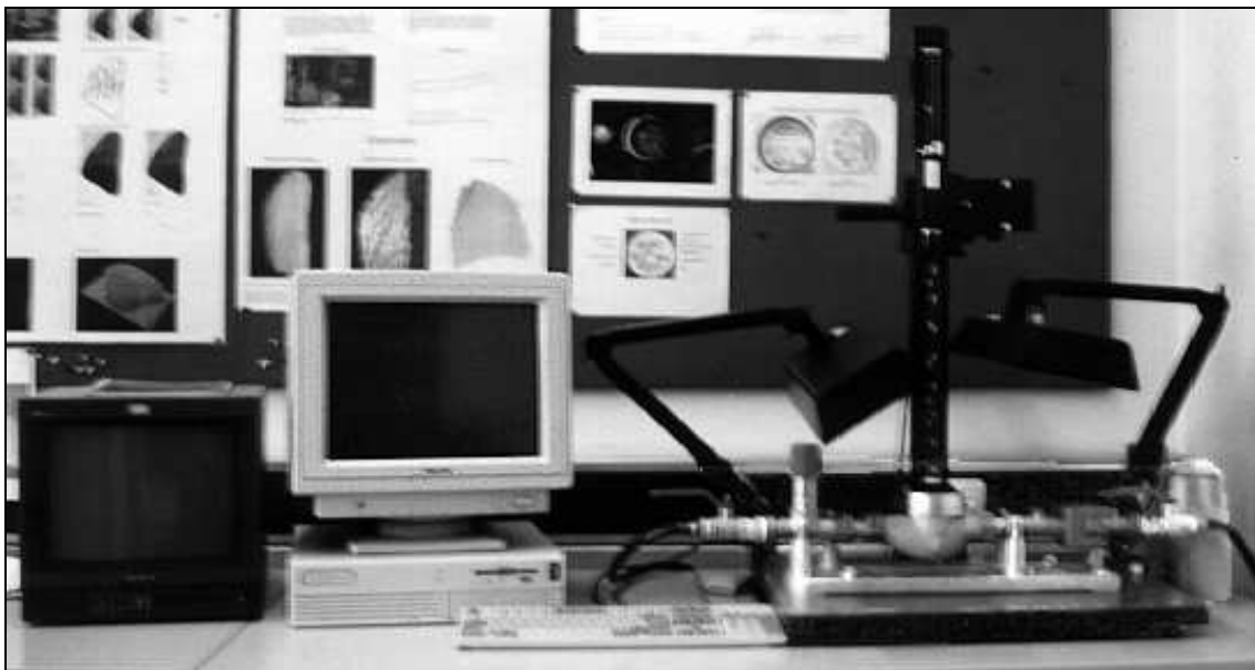
Figure 5.4 Laboratory setup showing camera, PC, and control monitor and preliminary illumination
