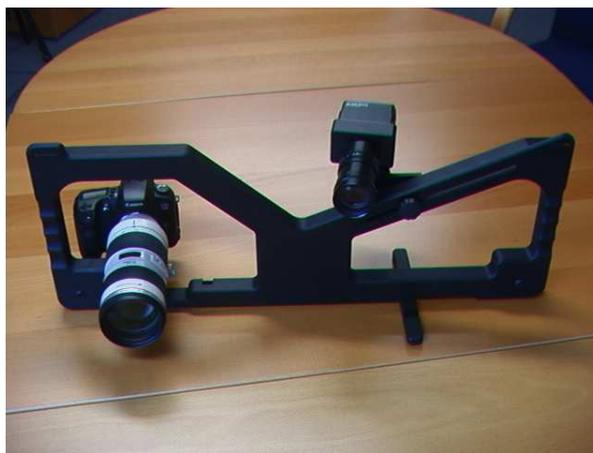
Figure 2: Eyetronic's ShapeCam consisting of a CCD-camera (left) and a slide-projector acting as flashlight mounted on the top-right part of the handling frame.
