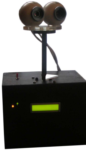
Figure 3.15: Image from the rotating Head, the figure shows a front view of the construction. The orange led indicates that the head is turned on and the green led changes its state (on/off) every time a command arrives from the computer. The LCD can be used to display information.
