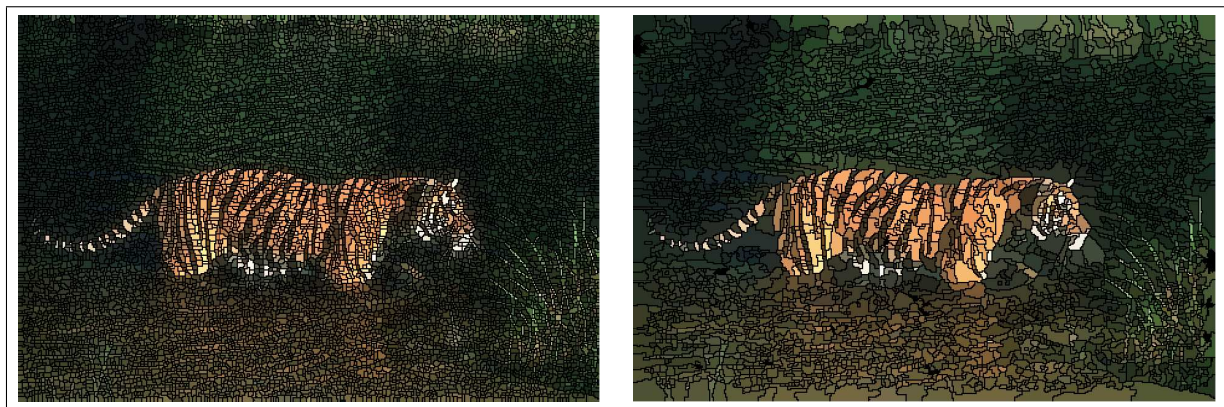
Figure 3: Example of Watershed segmentation based on symmetry maxima seeds (right) and without it, using only gradient minima (left). Note the number of segments on the right side is significantly lower than on the left side, but the segments on the right have still relatively low complex shapes in majority of cases.
